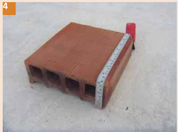
4 Tiles should be laid in order to allow ventilation through them for better performance. For this purpose at least 4 inch gap should be provided between open ends of hollow tiles and edge of roof.
